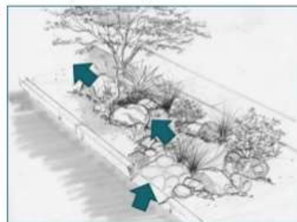
Rain garden and curb cuts capture, slow, and polish street runoff; may be paired with under drain to convey larger flows after polishing first-flush
